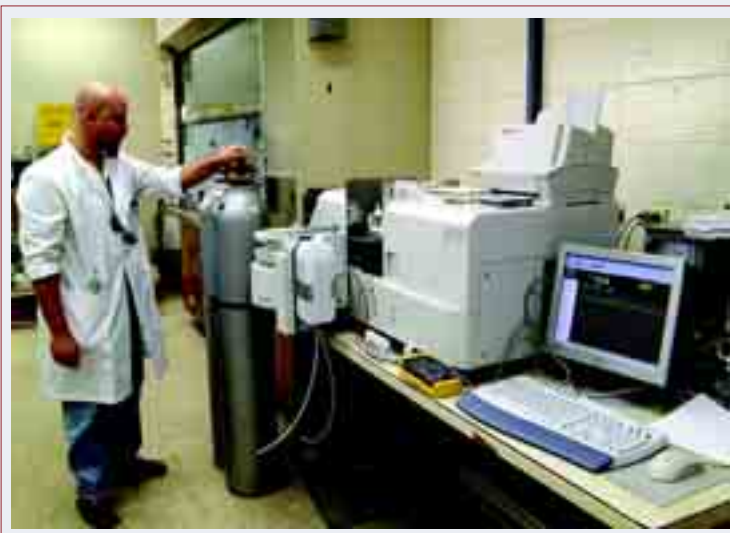
The newly acquired Shimadzu Atomic Absorption spectrophotometer was set up to analyze Si and Ca in samples of evaporator scale and mixed and clarified juices.
