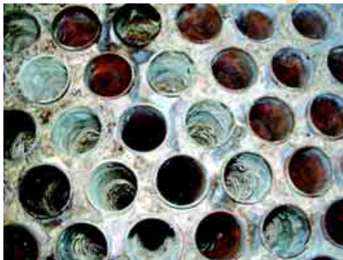
Figure 13. Scale in the final effect tubes and on the lower tubesheet at the St. James Sugar Mill.
