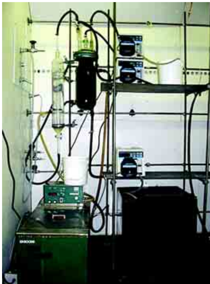
Figure 5. A 4L laboratory anaerobic reactor for dilute filter cake slurry.
